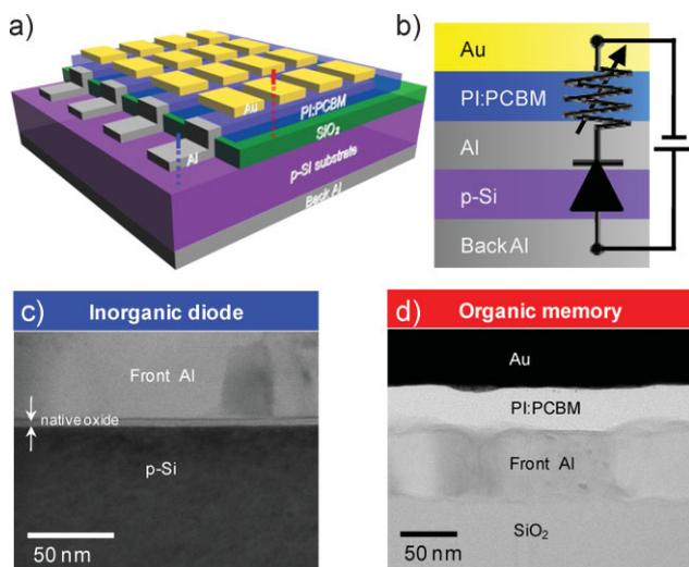
**Figure 1.** a) A schematic of 1D–1R hybrid-type memory devices. Blue and red lines indicate the inorganic Schottky diode (1D) component and the organic resistive memory (1R) component, respectively. b) A schematic of the layered structure and an electronic circuit diagram of the 1D–1R device. c) A TEM image of an inorganic Schottky junction diode (across the blue line in (a)). d) A TEM image of the organic memory (Al/PI:PCBM: Au) (across the red line in (a)).
