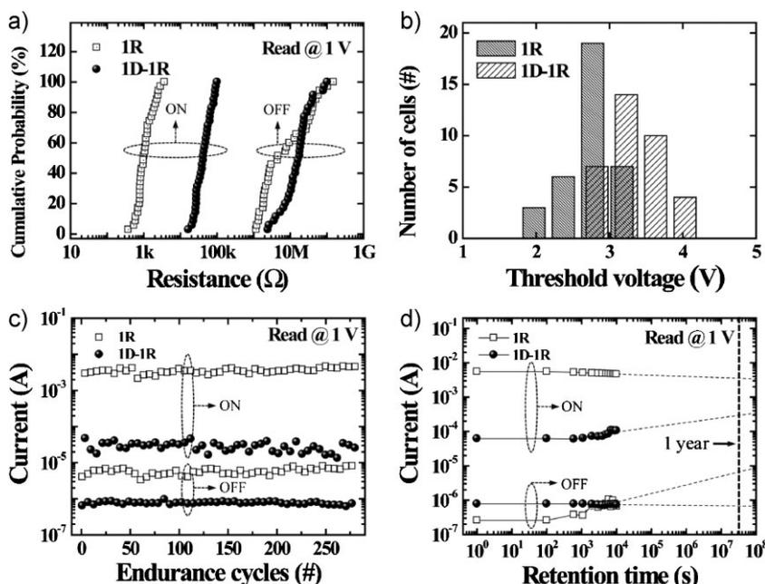
**Figure 3.** a) Cumulative probability data of each ON and OFF resistance for 1R and 1D–1R devices. ON and OFF resistances were measured at a voltage of 1 V. b) Comparison of the threshold voltage distributions of 1R and 1D–1R devices. c) Endurance cycles of 1R and 1D–1R devices. d) Retention times of 1R and 1D–1R devices. The extrapolated retention time can be estimated as more than 1 year.
