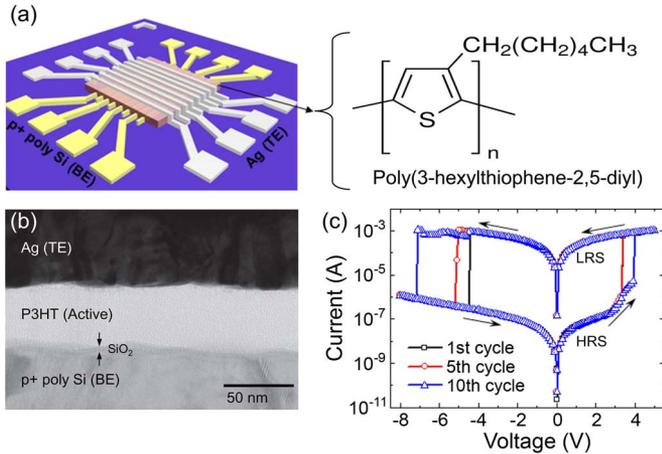
Fig. 1. (a) Schematic of P3HT-based organic memory devices with an  $8 \times 8$  array cell structure. (b) TEM image showing each layer of Ag/P3HT/p<sup>+</sup> poly-Si. (c)  $I$ - $V$  characteristics of an organic memory device.
