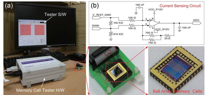
Fig. 3. (a) Optical image of the PC-interface memory cell tester used to independently address the data in the memory cells. At right, two enlarged images show that the organic devices are connected to a package embedded in a socket on a plastic IC chip. (b) Current-sensing circuit to read the resistance state of each memory cell.
