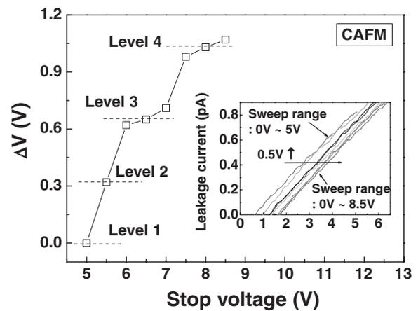
Fig. 3. Room temperature multi-level charge storage in silicon nanocrystals incorporated in silicon nitride at a gate area of  $100 \text{ nm}^2$ . The inset shows the  $I$ - $V$  measurement that was performed from 0V to different stop voltages.
