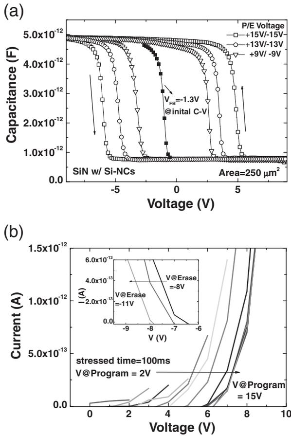
Fig. 1. (a)  $C$ - $V$  hysteresis curve of SiN with Si-NCs for different program/erase voltage and initial  $C$ - $V$  (b) shift of  $I$ - $V$  curve for different program voltage at a gate of  $100 \times 100 \mu\text{m}^2$ . Inset of (b) shows shift of  $I$ - $V$  curve for different erase voltages.
