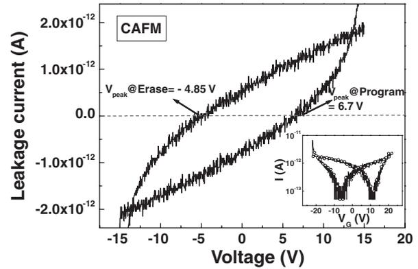
Fig. 2.  $I$ - $V$  hysteresis curve at a gate of about  $100 \text{ nm}^2$ .  $I$ - $V$  hysteresis was measured by C-AFM. The inset shows the absolute value.
