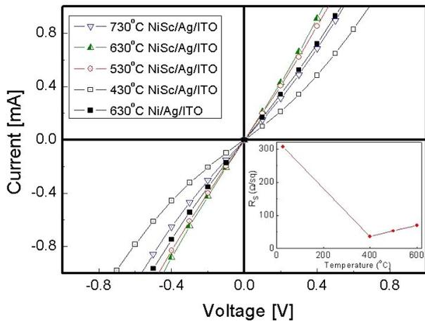
Fig. 1. Typical I-V characteristics of the NiSc/Ag/ITO and the Ni/Ag/ITO contacts as functions of the annealing temperature, as measured on 4- $\mu\text{m}$ -spaced pads.
