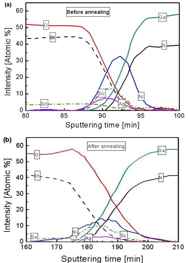
Fig. 2. AES depth profiles of the NiSc/Ag/ITO contacts (a) before and (b) after annealing at 630  $^\circ\text{C}$  for 1 min in air.
