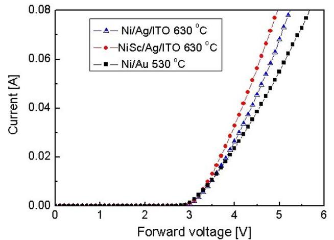
Fig. 4. I-V characteristics of near-UV LEDs (400 nm) fabricated using different *p*-type electrodes, all annealed for 1 min in air.
