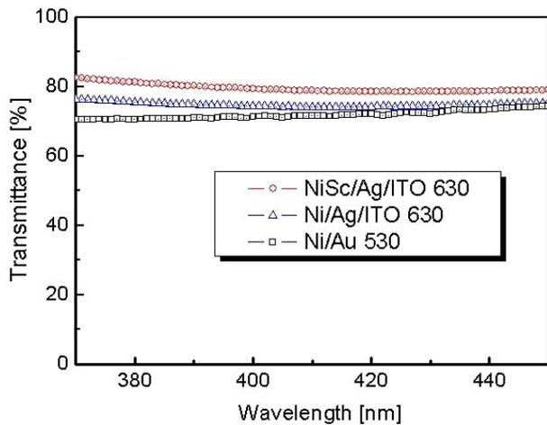
Fig. 3. Transmittance of the 630 °C-annealed NiSc/Ag/ITO, 630 °C-annealed Ni/Ag/ITO, and 530 °C-annealed Ni/Au contacts, all annealed for 1min in air.
