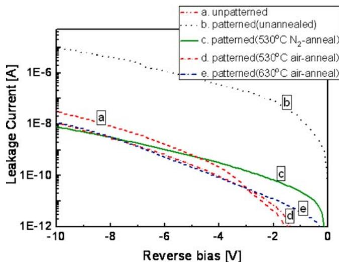
Fig. 3 (online colour at: [www.pss-a.com](http://www.pss-a.com)) Reverse leakage characteristics of LEDs made with the CIO/ITO p-contact layers before and after patterning.
