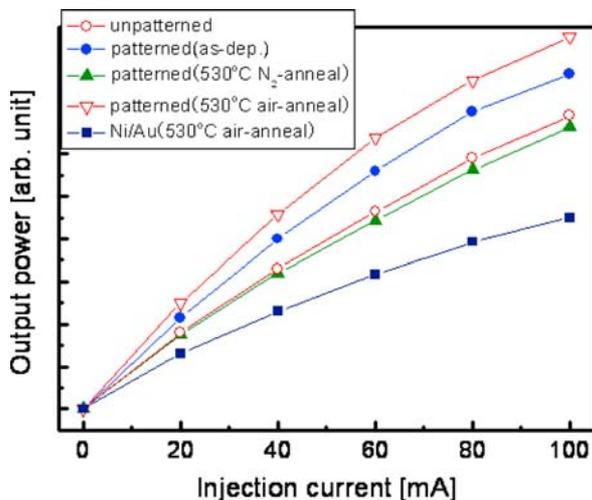
**Fig. 5** (online colour at: [www.pss-a.com](http://www.pss-a.com)) Light output–current ( $L-I$ ) characteristics of LEDs before and after patterning as a function of the forward drive current. It is shown that the patterned LEDs before and after annealing at 530 °C in air give much higher light output power compared to that of the unpatterned sample.
