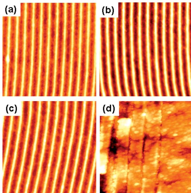
**Fig. 1** (online colour at: [www.pss-a.com](http://www.pss-a.com)) AFM images ( $5\ \mu\text{m} \times 5\ \mu\text{m}$ ) of the 1-D nano-patterned ITO layers. Annealed at  $530\ ^\circ\text{C}$  in either (a) air-ambient or (b)  $\text{N}_2$ -ambient; (c) unannealed; (d) annealed at  $630\ ^\circ\text{C}$  in air.
