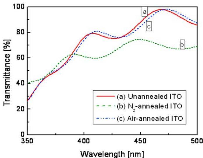
**Fig. 4** (online colour at: [www.pss-a.com](http://www.pss-a.com)) Transmittance of ITO films before and after annealing in either air or N<sub>2</sub> ambient.
