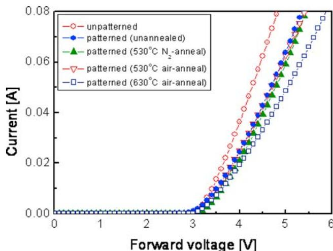
Fig. 2 (online colour at: [www.pss-a.com](http://www.pss-a.com)) Forward  $I$ - $V$  characteristics of LEDs fabricated with the CIO(3 nm)/ITO(400 nm) p-contact layers before and after patterning.
