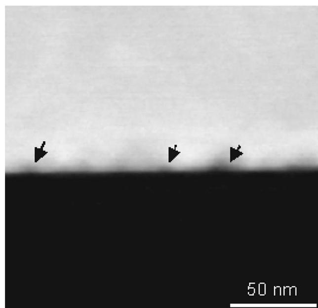
**Figure 3.** A cross-section STEM *z*-contrast image obtained from the ITO/Ag sample after annealing at 530°C.
