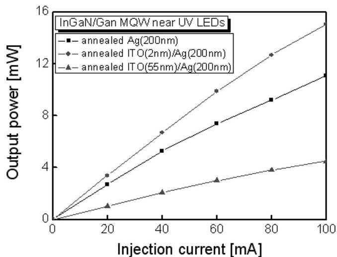
**Figure 5.** The light output-current ( $L$ - $I$ ) characteristics of the LEDs fabricated with the Ag ohmic reflectors with and without the ITO interlayers (annealed at 530°C) as a function of the forward drive current.
