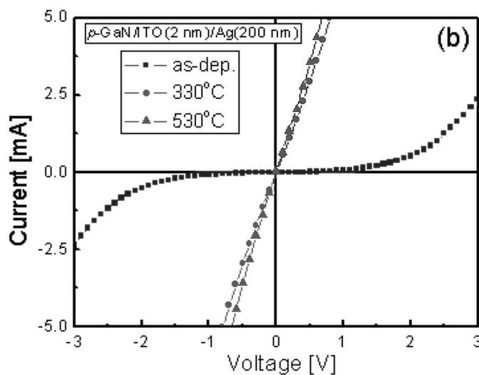
**Figure 1.** The typical *I-V* characteristics of (a) the ITO (55 nm)/Ag (200 nm) contacts and (b) the ITO (2 nm)/Ag (200 nm) contacts as a function of the annealing temperature. (c) Relation between the total resistance and the pad spacing, where  $R_o$  is the outer radius and  $R_i$  is inner radius.
