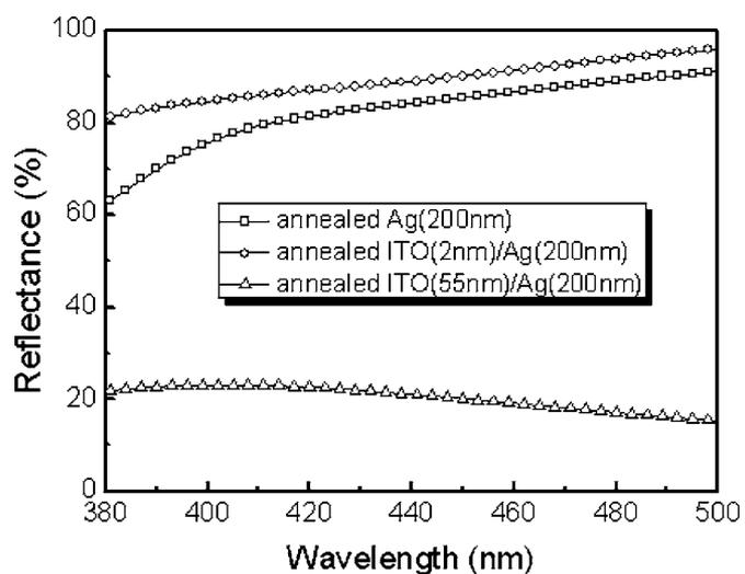
**Figure 2.** The light reflectance of the ITO (2 nm)/Ag (200 nm), ITO (55 nm)/Ag (200 nm), and single Ag (200 nm) contacts, which were annealed at 530°C.
