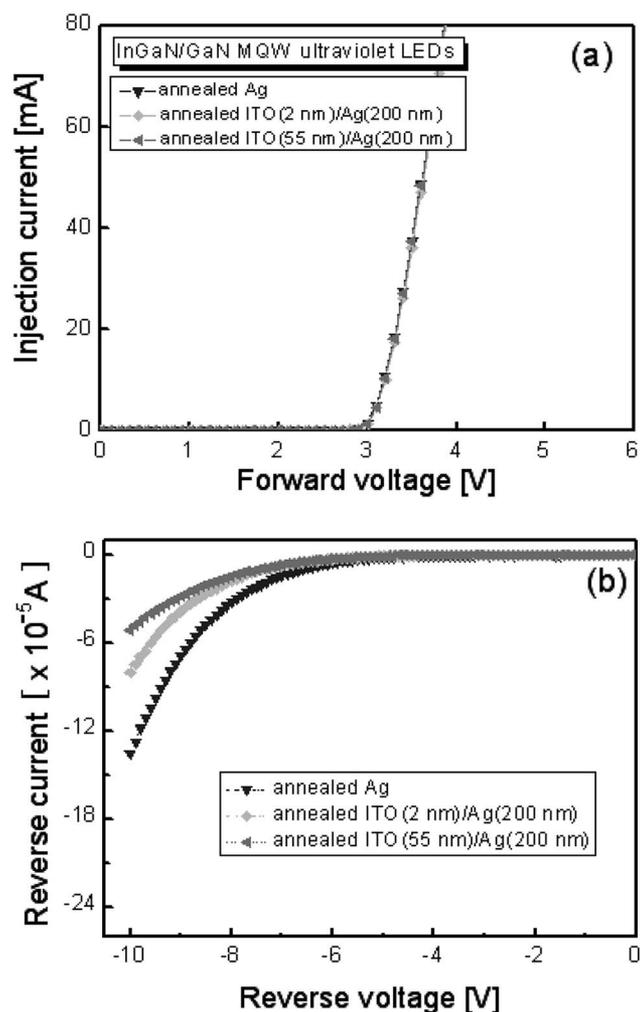
**Figure 4.** (a) Forward and (b) reverse electrical characteristics of near UV LEDs fabricated with the single Ag and ITO/Ag ohmic contacts, which were annealed at 530°C.
