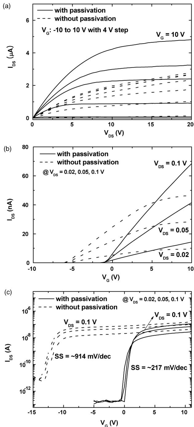
Fig. 3. (a) Source–drain current vs. voltage ( $I_{\text{DS}} - V_{\text{DS}}$ ) characteristics at different gate voltages with and without passivation, (b) source–drain current vs. gate voltage ( $I_{\text{DS}} - V_{\text{G}}$ ) characteristics at different source–drain biases for the same ZnO nanowire FET, respectively. (c) Logarithmic plot of  $I_{\text{DS}} - V_{\text{G}}$  curves at  $V_{\text{DS}} = 0.02, 0.05, \text{ and } 0.1 \text{ V}$  for another ZnO nanowire FET device.
