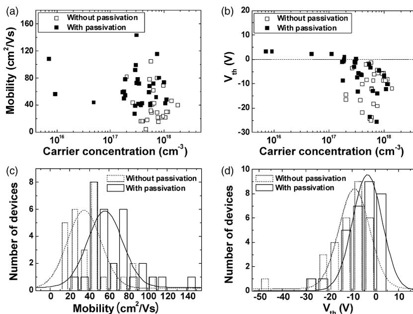
Fig. 4. (a) Mobility vs. carrier concentration and (b) threshold voltage ( $V_{\text{th}}$ ) vs. carrier concentration for all ZnO nanowire FETs fabricated. Histogram of threshold voltages (a) and mobility (b) for the ZnO nanowire FETs with and without passivation.
