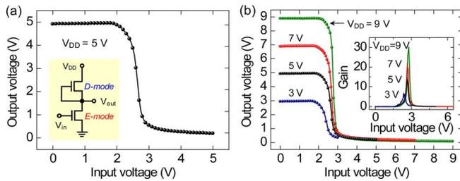
FIG. 3. (Color online) (a) VTC curve of a logic inverter composed of  $n$ -channel D-mode and  $n$ -channel E-mode ZnO nanowire FETs, obtained at  $V_{DD}=5$  V. The inset shows an inverter circuit diagram. (b) VTC curves of the inverter obtained under various values of  $V_{DD}$  from 3 to 9 V with a 2 V step. The inset shows voltage gain curves derived from the various VTC curves.
