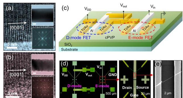
FIG. 1. (Color online) HRTEM images of (a) a smooth ZnO nanowire grown on Au-sapphire and (b) a corrugated ZnO nanowire grown on Au-GZO film. Insets show low magnification TEM images (upper) and computed fast Fourier transform patterns (lower). The scale bars are 20 nm in the upper insets. (c) Schematic illustration of logic inverter composed of D-mode and E-mode nanowire FETs. (d) Optical images of the fabricated inverters. (e) SEM image of a ZnO nanowire FET.
