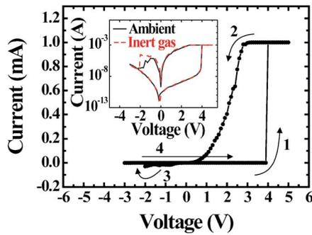
FIG. 2. (Color online)  $I$ - $V$  characteristics of a WPF-oxy-F memory device. Inset shows the semilog plot of the  $I$ - $V$  characteristics measured in ambient (black solid line) and inert gas condition (red dash line).
