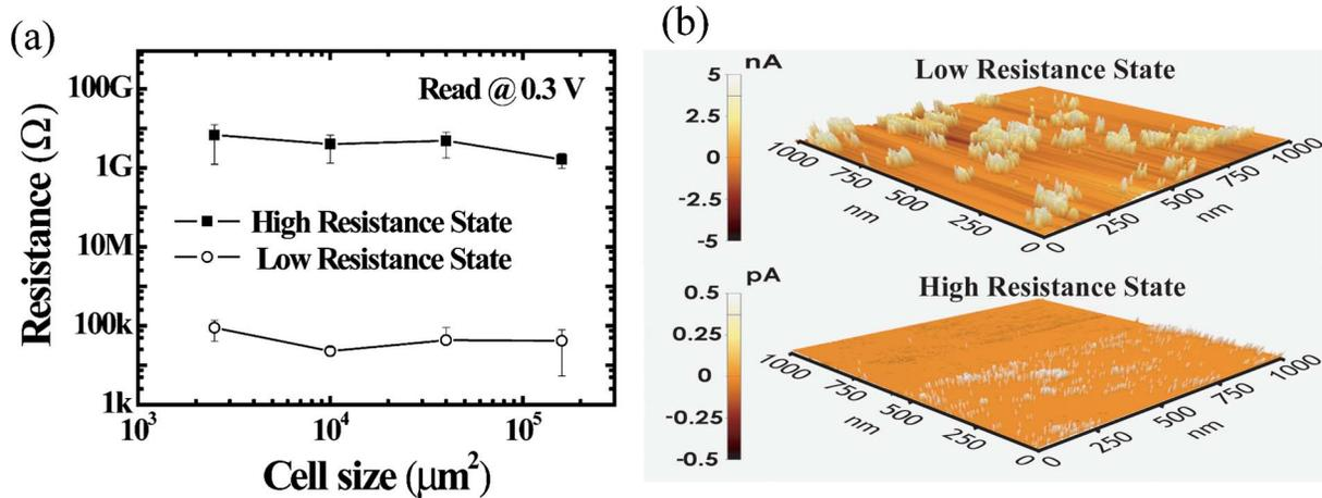
FIG. 4. (Color online) (a) Resistance values of two resistance states (HRS and LRS) of a WPF-oxy-F memory device as a function of the junction areas. (b) Current images of high and LRSs obtained by CAFM measurement.
