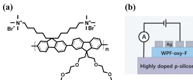
FIG. 1. (Color online) (a) Chemical structure of WPF-oxy-F polyfluorene derivative. (b) Schematic of single component WPF-oxy-F memory device.
