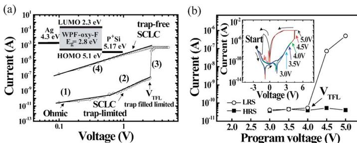
FIG. 3. (Color online) (a)  $I$ - $V$  characteristics of a WPF-oxy-F memory device in log-log scale. Inset figure shows energy band diagram of WPF-oxy-F memory device. (b) Programming voltage dependence of a WPF-oxy-F memory device. Excess bias ( $V_{\text{th}}$ ) required changing the resistance of WPF-oxy-F memory device from HRS to LRS. The inset figure shows stop voltage dependent  $I$ - $V$  characteristic.
