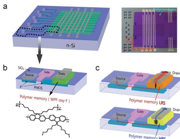
**Figure 1.** a) Schematic and optical image of 1T–1R hybrid devices. The area with the black dotted line indicates a silicon transistor (1T) and a polymer memory (1R). b) Schematic of a single 1T–1R device and chemical structure of WPF-oxy-F. c) Schematics of basic operation of the 1T–1R device. The current flow from source to drain in the 1T–1R device is controlled by the resistance state of the polymer memory device (see text).
