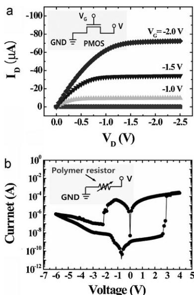
**Figure 2.** a)  $I_D$ - $V_D$  characteristics of the p-MOSFET device and its circuit diagram. b)  $I$ - $V$  characteristics of polymer memory device and its circuit diagram.
