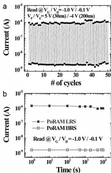
**Figure 4.** a) The endurance of the 1T–1R device with consecutive single voltage pulses applied to the polymer memory device. The measurement conditions are a  $5$  V pulse (writing process,  $V_P$ ) and a  $-4$  V pulse (erasing process,  $V_E$ ) with pulse duration ( $\tau_P$ ) of  $30$  and  $200$  ms, respectively. b) Retention characteristics of the 1T–1R device. The current value was read at a fixed gate of  $-1.0$  V and drain bias of  $-0.1$  V.
