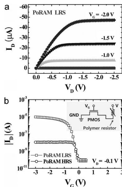
**Figure 3.** a)  $I_D$ - $V_D$  characteristics of the 1T-1R device. b)  $I_D$ - $V_G$  characteristics of the 1T-1R device with respect to the resistance state of polymer memory device.
