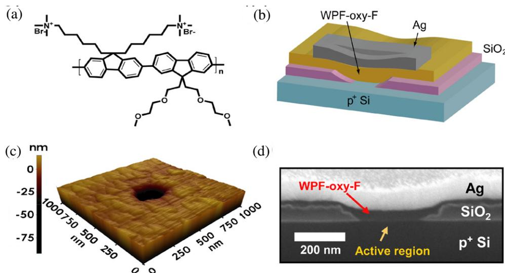
**Figure 1.** (a) Chemical structure of WPF-oxy-F polyfluorene derivative. (b) Schematic of a polymer memory device in a via-hole structure. (c) AFM image of a via-hole of area  $200 \times 200 \text{ nm}^2$ . (d) SEM image of a tilt view of a via-hole polymer memory device.
