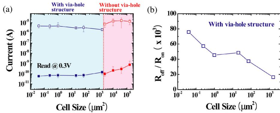
**Figure 3.** (a) Current values of the ON and OFF states of polymer memory devices as a function of active area. (b) Dependence of the OFF/ON resistance ratio of polymer memory devices as a function of active area.
