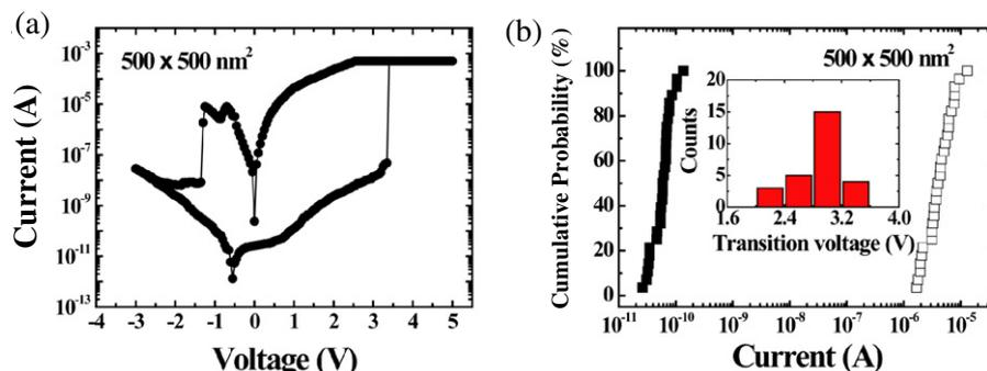
**Figure 2.** (a) Semilog scale  $I$ - $V$  characteristics of a polymer memory device with a  $500 \times 500 \text{ nm}^2$  via-hole. (b) A cumulative probability data set for polymer memory devices with a  $500 \times 500 \text{ nm}^2$  via-hole (28 devices), showing a good device-to-device switching uniformity. The inset figure shows the histogram of the OFF-to-ON transition for polymer memory devices with a  $500 \times 500 \text{ nm}^2$  via-hole.
