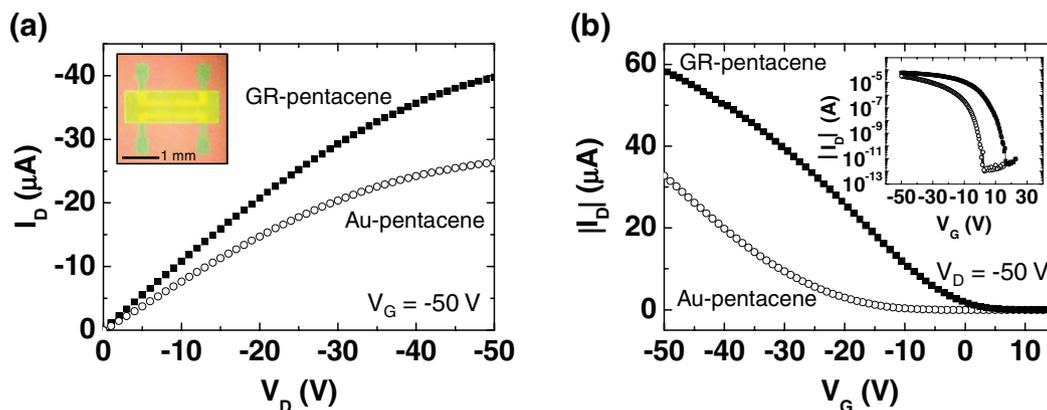
**Figure 2.** a)  $I_D$ - $V_D$  and b)  $I_D$ - $V_G$  characteristics of GR-pentacene and Au-pentacene OFETs with a channel length of 50  $\mu\text{m}$ . The inset in (a) is an optical image of a fabricated GR-pentacene OFET device. The inset in (b) shows the transfer characteristics on a semi-logarithmic scale.
