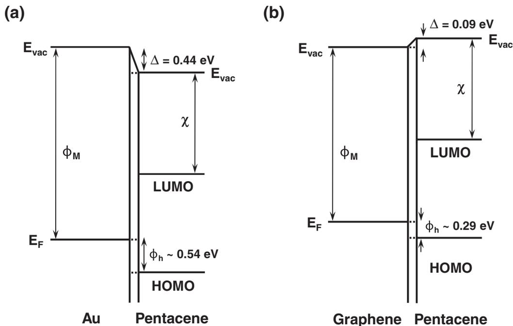
**Figure 5.** Schematic energy diagrams of a) the Au-pentacene and b) the GR-pentacene interfaces. The energy level alignments with the interfacial dipole barrier were determined by Kelvin-probe measurements. The hole-injection barrier ( $\Phi_h$ ), the electron affinity ( $\chi$ ), and the interfacial dipole barrier ( $\Delta$ ) are indicated in the diagrams.
