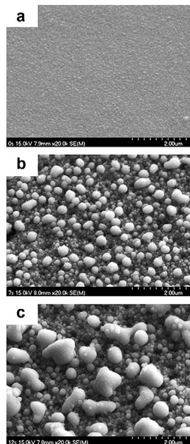
Fig. 3. SEM images obtained from (a) the post-annealed ITO layer (etched for 0 s), (b) the post-annealed ITO layer (etched for 7 s), and (c) the post-annealed ITO layer (etched for 12 s).
