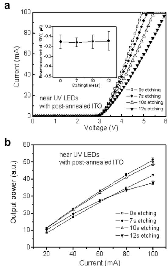
Fig. 2. (a) The typical  $I$ – $V$  characteristics of near-UV LEDs fabricated with the post-annealed ITO electrodes. The inset shows a variation of reverse current at  $-10$  V for the LEDs with the post-annealed ITO layers. (b) The light output–current ( $L$ – $I$ ) characteristics of LEDs fabricated with the post-annealed ITO layers.
