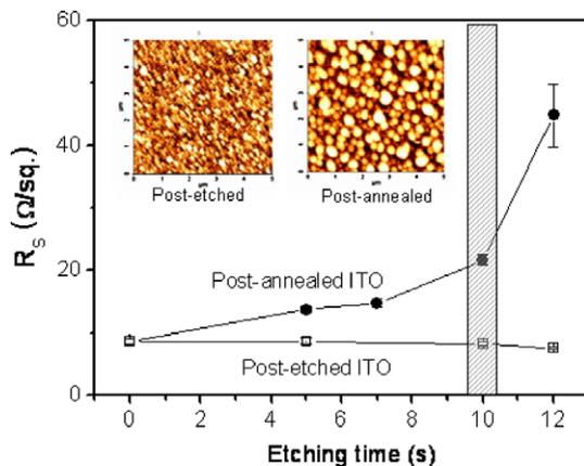
Fig. 1. Plots of the sheet resistances for the ITO layers as a function of the etching time. AFM images of the ITO layers are shown in the inset.
