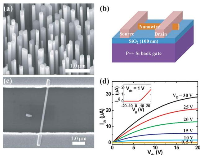
FIG. 1. (Color online) (a) FESEM image of grown ZnO nanowires. (b) Schematic of a ZnO nanowire FET. (c) FESEM image of a ZnO nanowire across metal electrodes. (d) Typical  $I_{ds}$ - $V_{ds}$  curves for different gate biases from 0 to 30 V with 5 V step. The inset is  $I_{ds}$ - $V_g$  curve measured at  $V_{ds}=1$  V.
