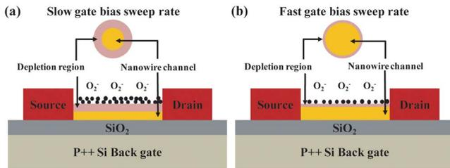
FIG. 3. (Color online) Schematics illustrating the effect of gate bias sweep rate. A larger depletion region is formed with slower gate bias sweep rates (a) than the case for faster gate bias sweep rate (b).
