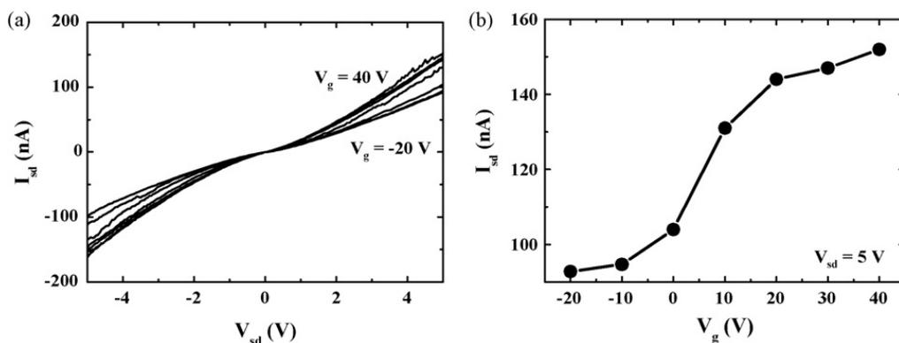
Fig. 7. (a)  $I_{sd}$ – $V_{sd}$  plot for different gate biases from –40 to 20 V with 10 V increments for a VO<sub>2</sub> nanowire device. (b)  $I_{sd}$ – $V_g$  plot at a fixed  $V_{sd} = 5$  V.
