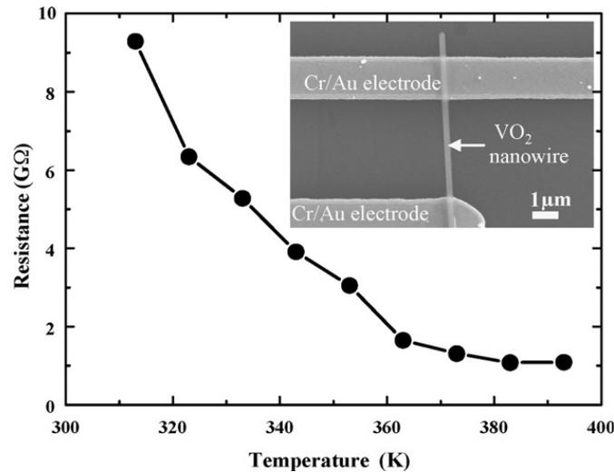
Fig. 6. Resistance of VO<sub>2</sub> nanowire as a function of temperature. Inset shows SEM image of a VO<sub>2</sub> nanowire electronic device.
