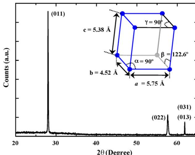
Fig. 2. XRD pattern of VO<sub>2</sub> nanowires. Inset is a schematic of a unit cell of VO<sub>2</sub> nanowires.
