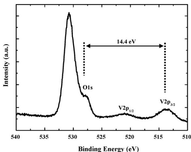
Fig. 4. XPS data of O 1s and V 2p spectra in VO<sub>2</sub> nanowires grown on Si<sub>3</sub>N<sub>4</sub>/Si substrate.
