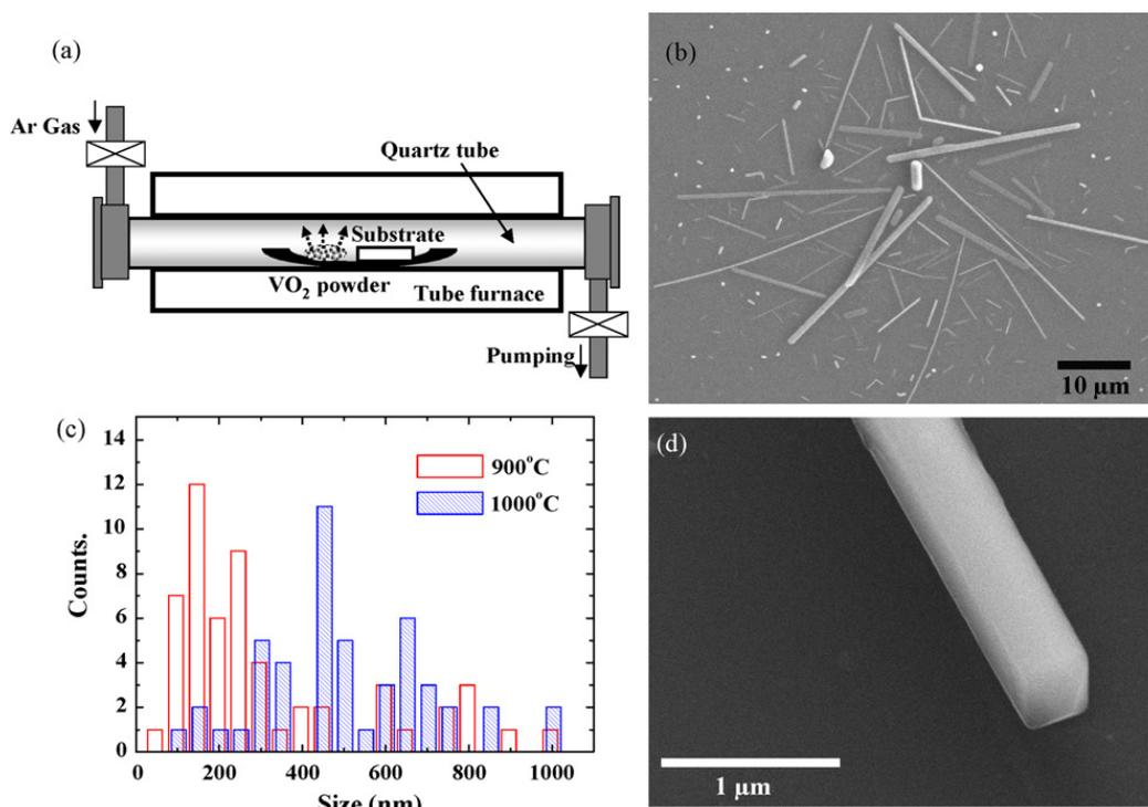
Fig. 1. (a) Schematic diagram of nanowire growth reactor. (b) SEM image of  $\text{VO}_2$  nanowires grown at  $900^\circ\text{C}$  on  $\text{Si}_3\text{N}_4/\text{Si}$  substrate. (c) Histogram of size and length of the nanowires grown at  $900^\circ\text{C}$  and  $1000^\circ\text{C}$ . (d) SEM image showing nanowire in a rectangular shape.
