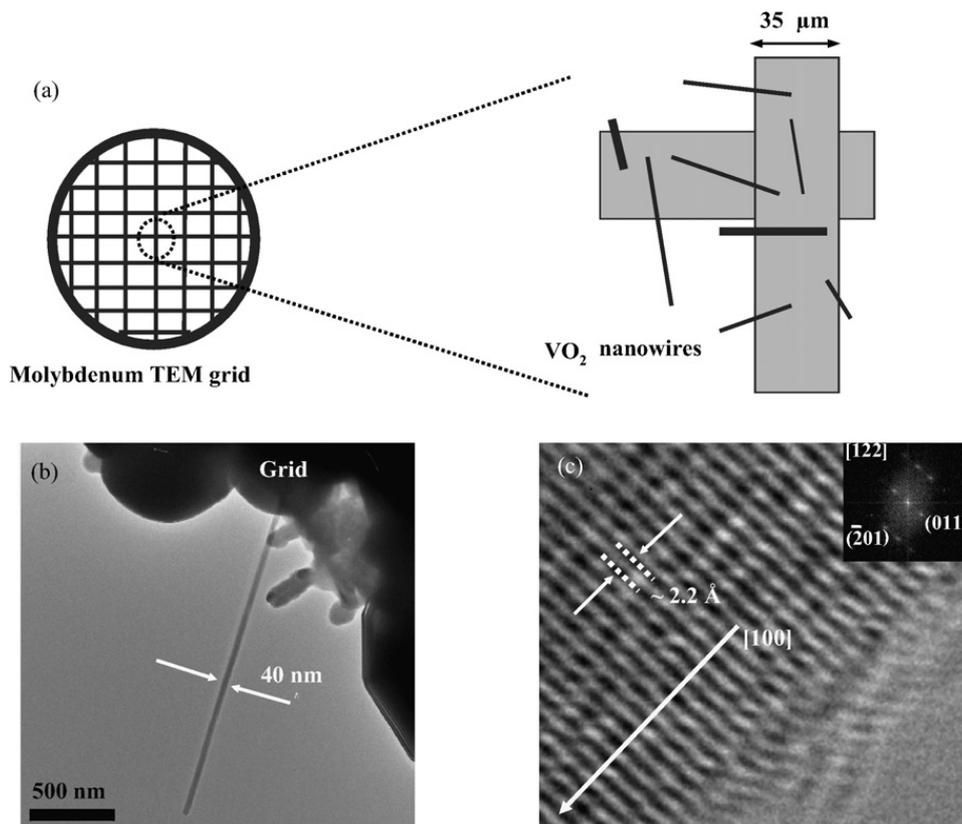
Fig. 5. (a) Schematics illustrating growth of VO<sub>2</sub> nanowires on Si<sub>3</sub>N<sub>4</sub> deposited molybdenum TEM grid. (b) TEM image of VO<sub>2</sub> nanowire ~40 nm in size. (c) HRTEM image of a nanowire with a fast Fourier transform image (inset). Interplanar lattice spacing is 2.2 Å in ( $\bar{2}01$ ) planes.
