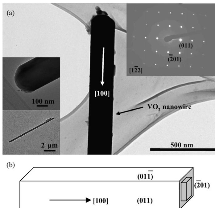
Fig. 3. (a) TEM images of a detached VO<sub>2</sub> nanowire. The insets are an electron diffraction pattern along the  $[1\bar{2}2]$  zone axis and low-magnification TEM images of the growth front and the whole VO<sub>2</sub> nanowire. (b) The structure schematic of the grown VO<sub>2</sub> nanowire.
