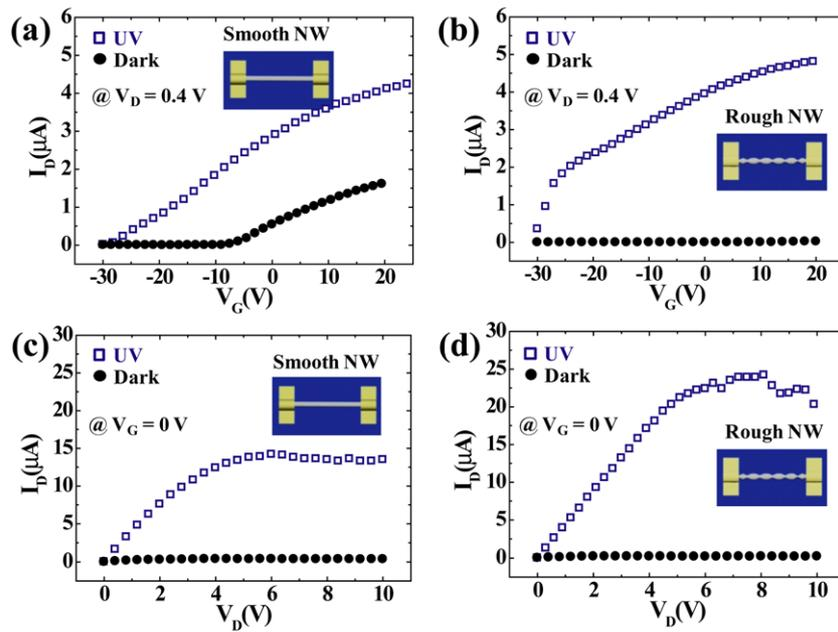
**Figure 2.** The electrical characteristics of ZnO NWs in the absence of light and under UV illumination. The insets display schematic images of smooth and rough ZnO NW FETs.  $I_D$ - $V_G$  (at  $V_D = 0.4$  V) and  $I_D$ - $V_D$  (at  $V_G = 0$  V) curves of smooth ((a), (c)) and rough ZnO NW FETs ((b), (d)), respectively.
