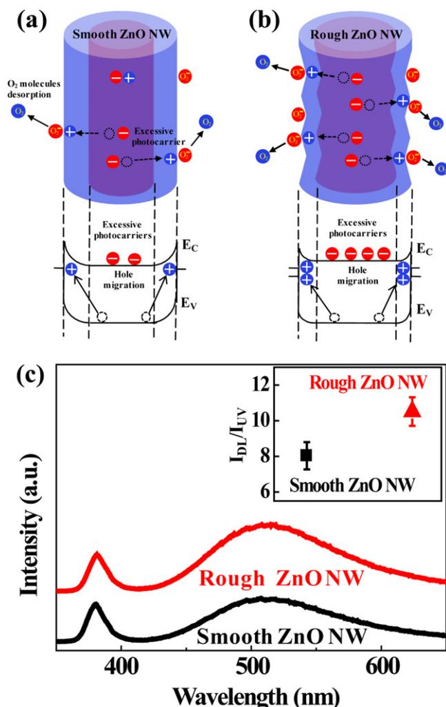
**Figure 5.** (Top) Schematic illustration of the mechanism of photocarrier generation and (bottom) the corresponding energy band diagrams of (a) smooth and (b) rough ZnO NWs under UV illumination.  $E_C$  is the conduction band and  $E_V$  is the valence band of ZnO NWs. (c) PL spectra of smooth (black line) and rough ZnO NWs (red line). To allow for clear comparison, the red line was shifted vertically. The inset displays the PL intensity ratios ( $I_{DL}/I_{UV}$ ) for two cases.
