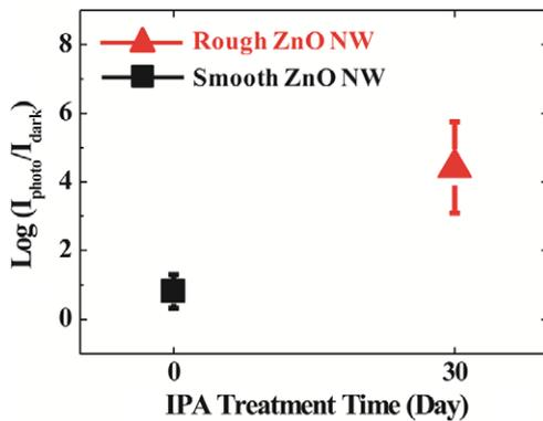
**Figure 3.** The statistical results of  $\log(I_{\text{photo}}/I_{\text{dark}})$  versus IPA treatment time for unmodified (smooth) and IPA-treated (rough) ZnO nanowire FETs obtained from the transfer characteristics of a total of eight devices. The currents measured at  $V_D = 0.4$  V and  $V_G = 0$  V were used to determine the  $I_{\text{photo}}/I_{\text{dark}}$  ratio.
