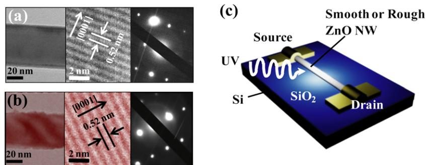
**Figure 1.** Low-magnification TEM images (left), HRTEM images (middle) and electron diffraction patterns (right) of (a) an unmodified ZnO NW and (b) a ZnO NW submerged in IPA for 30 days. (c) A schematic illustration of a ZnO NW FET under UV illumination.
