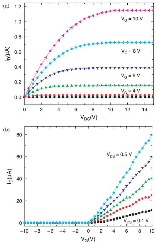
**Fig. 3.**  $I_D - V_{DS}$  characteristics (a) and  $I_D - V_G$  characteristics (b) of bottom-gate ZnO nanowire FET.
