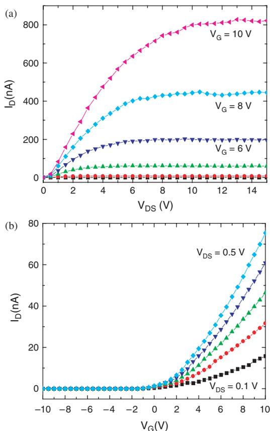
**Fig. 4.**  $I_D - V_{DS}$  characteristics (a) and  $I_D - V_G$  characteristics (b) of top-gate ZnO nanowire FET with a polymer gate dielectric layer.
