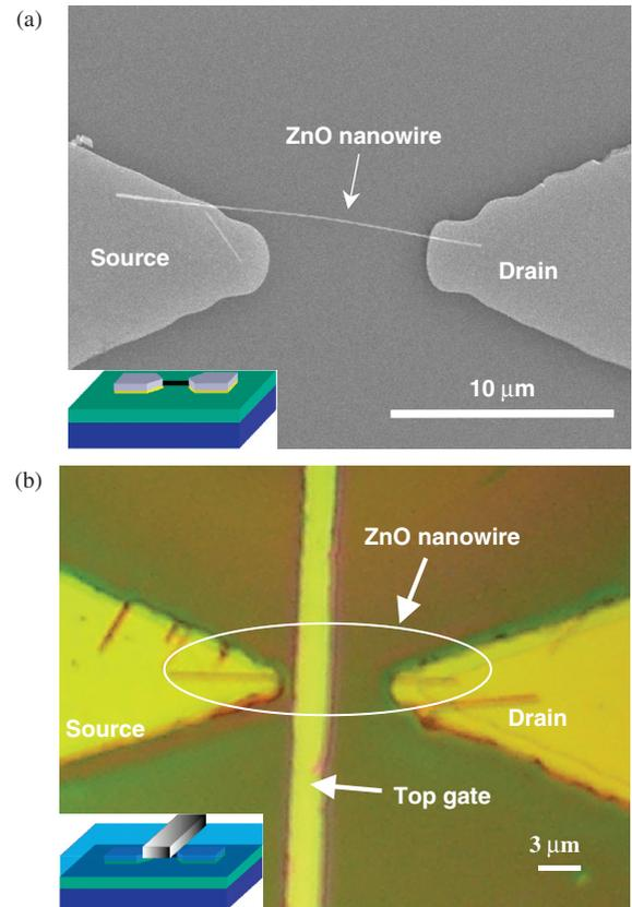
**Fig. 2.** (a) SEM image of assembled ZnO nanowire in bottom-gate configuration. (b) Optical microscope image of top-gate ZnO nanowire FET with a polymer gate dielectric layer.
