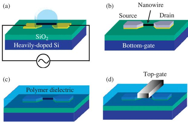
**Fig. 1.** Schematic diagrams of experimental procedure. (a) Direct assembly of nanowires by the dielectrophoresis method, (b) second metallization for source and drain electrodes, (c) deposition of a polymer gate dielectric layer, (d) fabrication of top-gate electrode. Bottom-gate configuration (b) and top-gate configuration (d).
